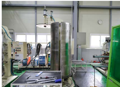
Vertical Assembly Fixture
