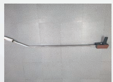
Thermometer For Melting Temperature Inspection
