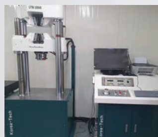
Universal Test Machine For Measuring Tensile Strength
